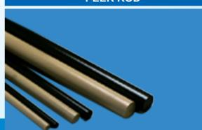
**PEEK (Poly Ether Ether Ketone)** is a high performance engineering thermoplastic that offers chemical and water resistance similar to PPS, but can operate at higher temperatures. PEEK can be used continuously to 480°F (250°C) and in hot water or steam without permanent loss in physical properties. For hostile environments, PEEK is a high strength alternative to fluoropolymers. PEEK carries a V-0 flammability rating and exhibits very low smoke and toxic gas emission when exposed to flame.
